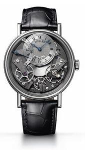
Nor does the new reference 7097 lag behind when it comes to the latest technology. Its 40mm case houses a movement with an inverted in-line lever escapement with silicon pallets and a silicon Breguet overcoil balance spring that ensure exceptional stability of rate.
